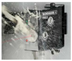
The Renishaw TRS2 is a replacement for the original TRS1 unit, which has been successfully installed on machines worldwide. With enhancements made to Renishaw's unique ToolWise™ technology, the TRS2 benefits from improved tool detection reliability and reduced cycle times.
