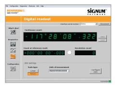
All Renishaw **SiGNUM**" encoders can connect via USB to a PC, where comprehensive **SiGNUM**" software enables optimum set-up and real-time system diagnostics, even when in full servo loop control. Si-FN adds a fully-functional DRO (digital readout) for further diagnostics.
