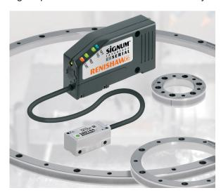
Si-FN interfaces are available with three resolution options. 'Normal' offers 20 bit resolution (0.0003 degree resolution) and speeds up to 4,500 rev/min; 'High Type A' has 23 bit resolution (0.000043 degree resolution), and 'High Type B' interfaces provide up to 26 bit resolution (0.0000054 degree resolution) for the highest precision while still achieving 600 rev/min.
