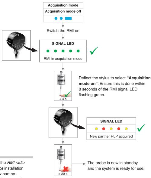
**NOTE:** Refer to the *RMI radio* machine interface installation guide (Renishaw part no. H-4113-8554) when partnering the RLP40.
