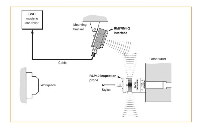
Radio transmission does not require line-of-sight between the probe and interface as it will pass through very small gaps and machine tool windows. This allows easy installation, either inside or outside the machine enclosure.
