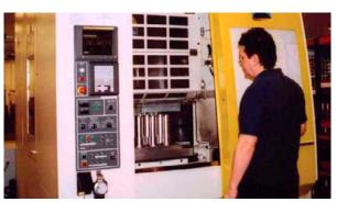
Machining centres, equipped with job set-up probes can now run batches of multiple components
