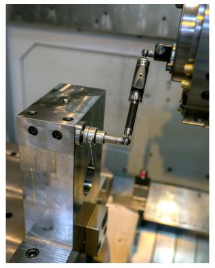
FMC Technologies uses Renishaw's QC20-W wireless ballbar to check the accuracy of its CNC machine tools
