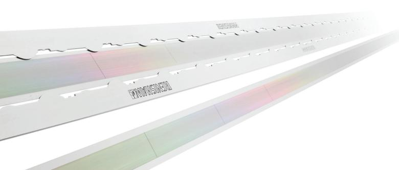
RTLC 20 or 40 µm linear encoder tape scale combines ±5 µm/m accuracy with the ruggedness of stainless steel. Two versions are available: self-adhesive RTLC-S and RTLC for use with the revolutionary *FASTRACK*™ track system from Renishaw.
