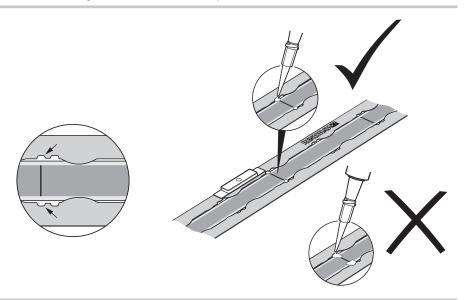
**NOTE:** Only apply Loctite 435 in these gaps to ensure the best bond. Loctite 435 will wick under the scale to lock it to the substrate.
