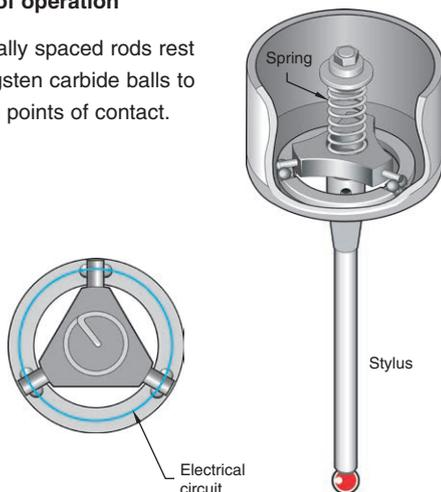
Under load of the spring, contact patches are created between the balls and the rods through which the electrical current flows. Upon making contact with (touching) a work-piece, the force translated through the stylus moves the balls and rods apart thus reducing the size of the contact patches and increasing their electrical resistance.
