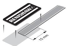
**CAUTION:** Ensure that excess epoxy is wiped away from the scale as it may affect the readhead signal level.
