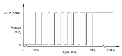
Between 50% and 70% the signal level  $V_x$  is a duty cycle. Time spent at 3.3 V increases with incremental signal level. At > 70% the signal level  $V_x$  is nominal 3.3 V.
