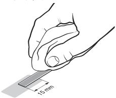
2. Thoroughly mix up a sachet of RGG-2 two-part epoxy adhesive and apply a small amount to the underside of the end clamp.
