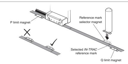
Apply firm finger pressure to the magnet via a clean, dry, lint-free cloth to ensure complete adhesion
