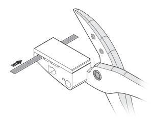
Hold the scale in place and close the shears in a smooth motion to cut through the scale.
