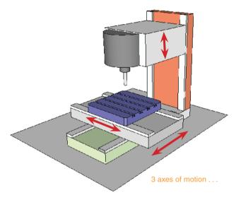
... and multiple potential positioning errors on each axis (and between axes)
