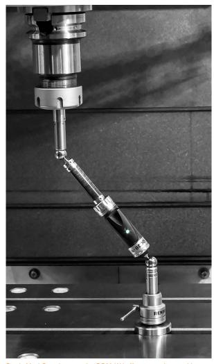
StankoMachComplex uses the QC20-W ballbar to monitor machine tool condition
