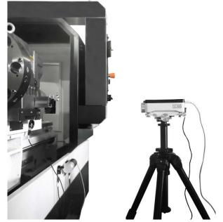
Checking accuracy of movements in machine tools with XL-80 laser system
